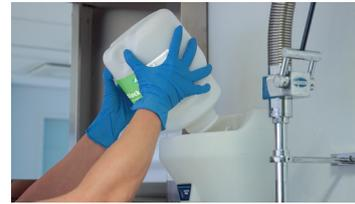
Remove the lid from the new block. It can easily be removed by lifting it in one side.
